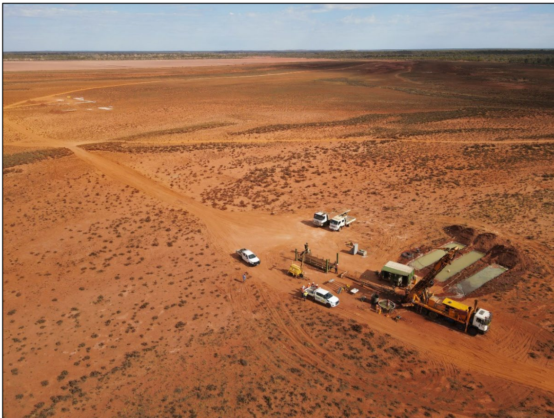
Figure 7. Diamond drilling at Kanowna East
