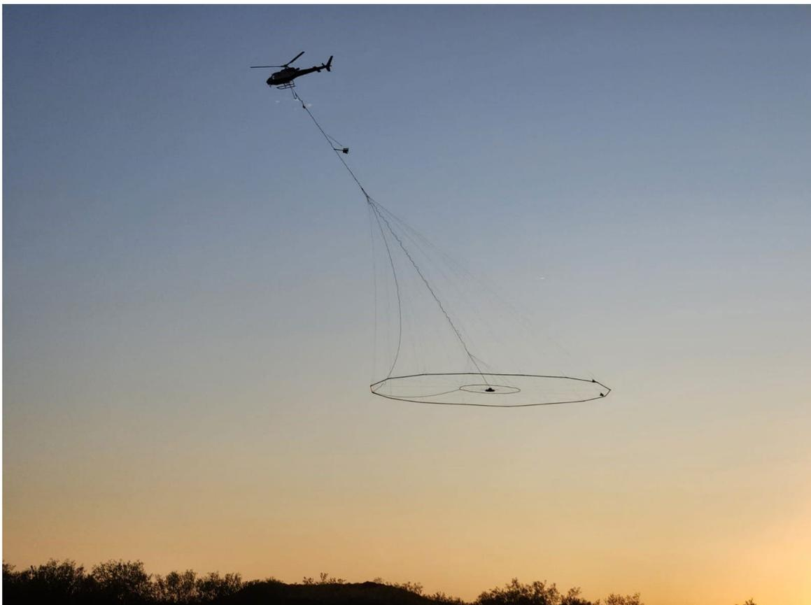
Figure 1. VTEM Max system in operation - Image courtesy of UTS Geophysics (Geotech)
