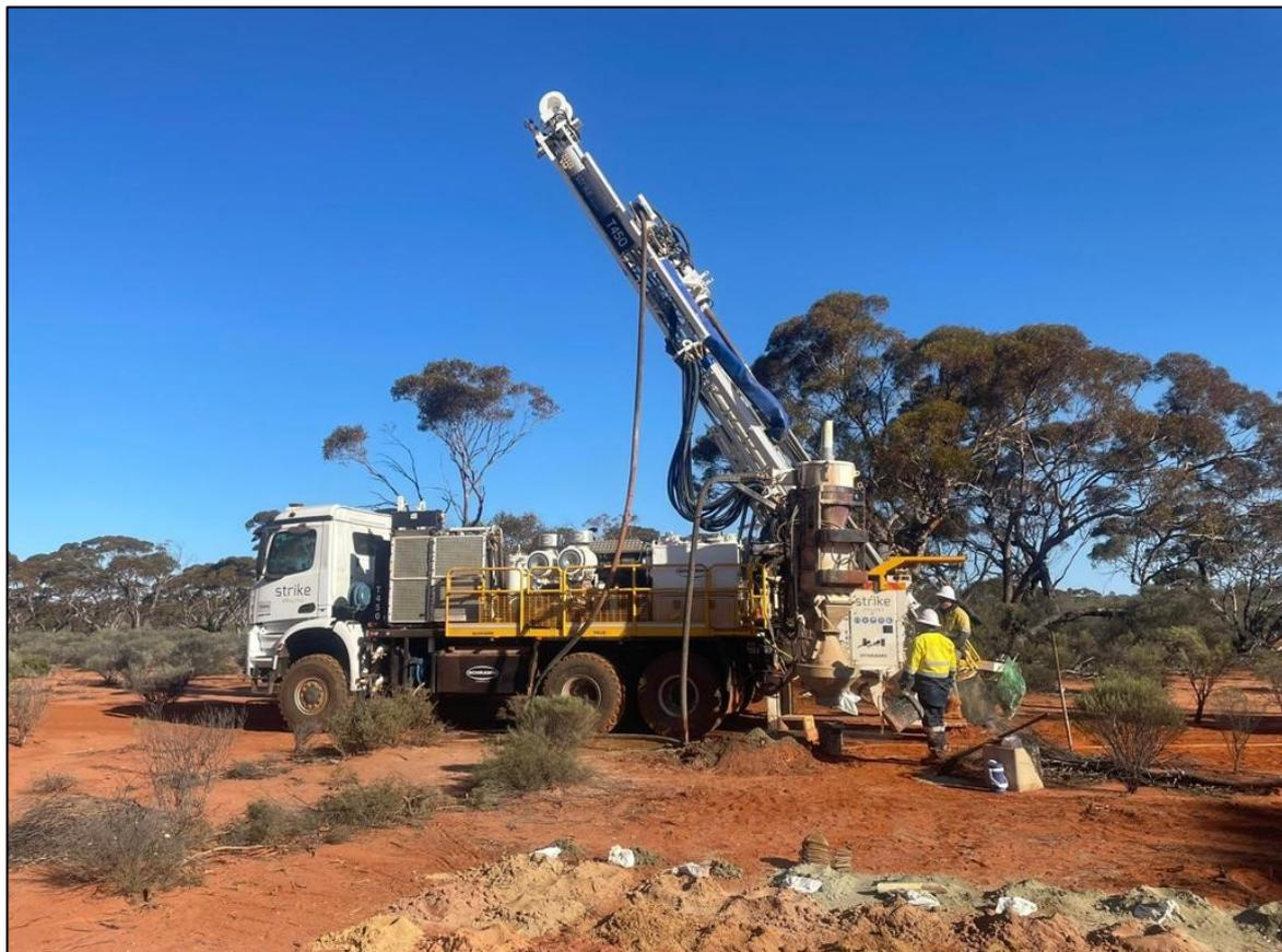
Figure 1. Aircore Drilling at Emu Lake
