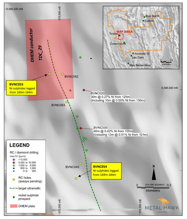
Figure 1. RC drilling at Torana – new highlights shown in yellow (assays pending)
