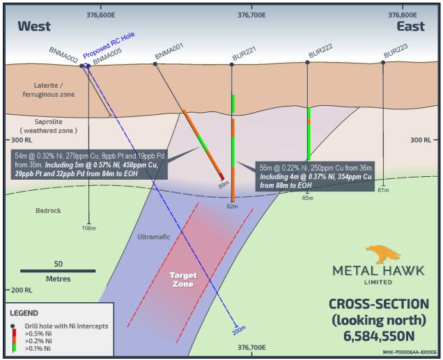
Figure 5. Berehaven Nickel Project simplified cross-section
