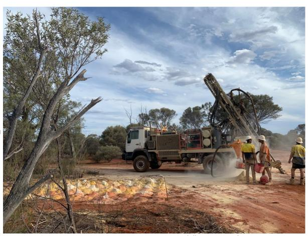
Figure 1. KTE Mining Services Aircore drill rig at Emu Lake
